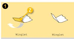
If there are Winglets, assemble as follows: For each Winglet, fold along the (Z) line, such that the winglet is upright at a 45-degree angle outwards from the wing.
